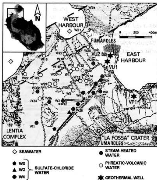
Figure 1. Map of Vulcano Porto area and location of studied well waters. The latter are subdivided in three groups as defined later on in the text. The dashed lines represent main structural lineaments (Gabbianelli et al. 1991).
